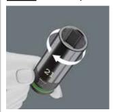
The rotating plastic sleeve allows for higher control during screwdriving. In addition, the surface of the rim is protected. The plastic sleeves are interchangeable.
