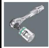
The Zyklop Mini 3 ratchet is the ideal tool for screwdriving in confined spaces. The fine toothing (60 teeth) allows a very low return angle of only 6°; the knurled wheel allows fast screwdriving even when there is no room for pivoting movement.
