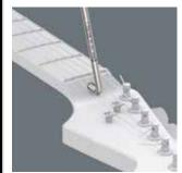
The special Hex-Plus geometry of the angle wrench makes for a better fit of the tool in the screw, reducing the risk of slippage and damage, and significantly improving the power transmission.
