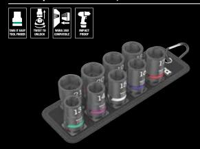
9-piece; robust textile socket belt, including snap hook to enable secure fastening to a belt loop or pocket. Non-woven reverse side and hook and loop strips for simple attachment e.g. to a wall, shelf, tool trolley and to the Wera 2go tool transport system. Fast and easy Twist to Unlock mechanism for secure storage and simple removal of the sockets.
