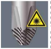
It happens time and time again that the tip slips out of the screw head when screwdriving, sometimes damaging valuable surfaces or even causing injury. The tips of the Wera Lasertip screwdrivers are microscopically roughened by means of a laser. This rough surface literally "bites" itself firmly into
