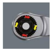
The dual-ratchet-teeth design means that a 76 fine-toothing division can be achieved from the 38 robust teeth with a return angle of only 4.7°.
