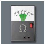
The electric surface resistance of the Wera ESD material is ≤ 10<sup>9</sup> ohm. This securely protects components against electrostatic energy and associated damage.
