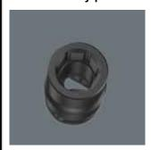
The hexagon profile allows the transmission of high forces and puts less strain on the edges of bolts or screw heads than a double hexagon profile. Finetoothed ratchets also make the use of a double hexagon profile superfluous, even in confined spaces, thanks to their small back-pivoting angle.
