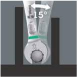
The Joker 6003 ring spanner with its special mouth geometry – a mouth side pivoted by 7.5° and the double hexagon geometry - doubles the placement possibilities when repeatedly turning the wrench 180° around the longitudinal axis. Bolts and
