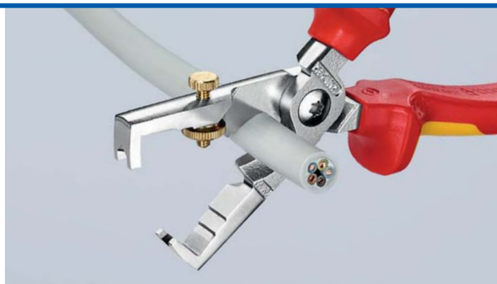
Induction hardened shear blade with precisely ground cutting edges for crushing-free cutting of copper cables of up to Ø 15 mm (5 x 2.5 mm 2 )
